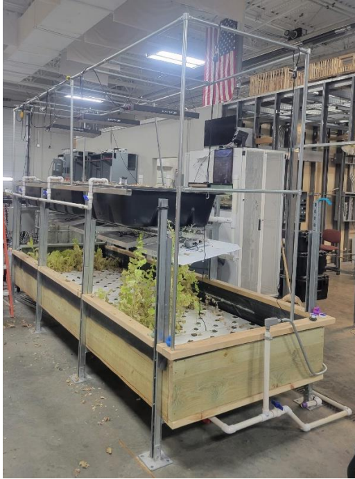
Media beds (upper) and raft beds (lower) in the aquaponics system
